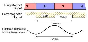
$V_{PROC}$  = the processed analog signal of the sinusoidal magnetic input
