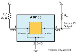
**Figure 2: Typical Application Circuit**
