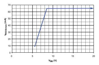
Figure 3. Current Capability of the 5 V Regulator (VREG5)
