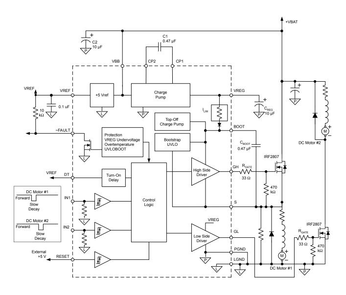
Diagram B. Independent drivers. One high-side drive and one low-side drive.
