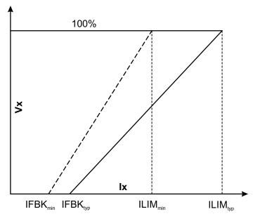
Figure 4: LDO Foldback Characteristics
