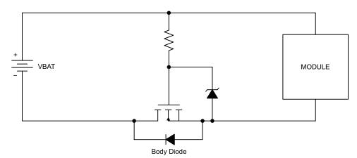
Functional Block Diagram Using an NMOS FET for Reverse-Battery Protection Instead of a Series Schottky Diode (D<sub>IN</sub>)
