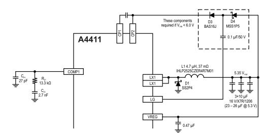
Functional Block Diagram Modifications for Buck Only Mode, f<sub>OSC</sub> = 2 MHz
