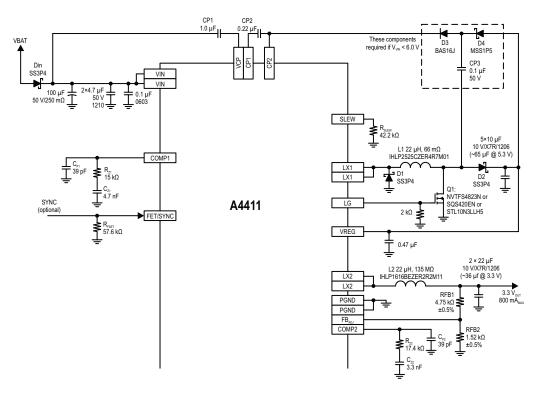
Functional Block Diagram Modifications for Buck-Boost Mode (f<sub>OSC</sub> = 400 kHz)
