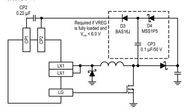
Figure 9: Charge pump enhancement components D3, D4, and CP3 are required if  $V_{VIN}$  < 6 V.
