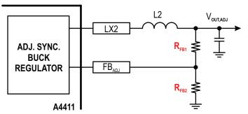
Figure 21: Setting the Synchronous Buck Output
