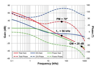
Figure 22: Bode Plot for the Sync. Buck at 3.3  $\rm V_{OUT}$
