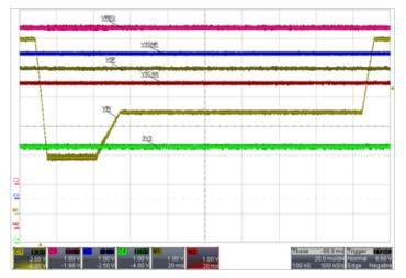
Figure 1: Buck-Boost Performance with Relatively Fast V<sub>VIN</sub> Transition Times for a Representative Start/Stop Waveform
