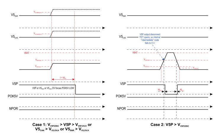
Figure 15: Overvoltage Cases for V5P, V5<sub>SNR</sub>, and V5<sub>CAN</sub>
