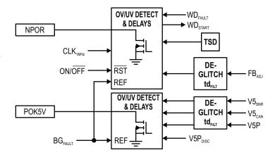
Figure 10: Fault Reporting Circuit
