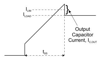
Figure 19: Output Current (I<sub>CO</sub>) During Startup
