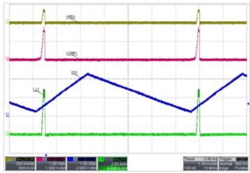
Figure 2: Pre-Regulator Hiccup Mode Operation when VREG is Shorted to GND and  $C_{SS1}$  = 22nF
