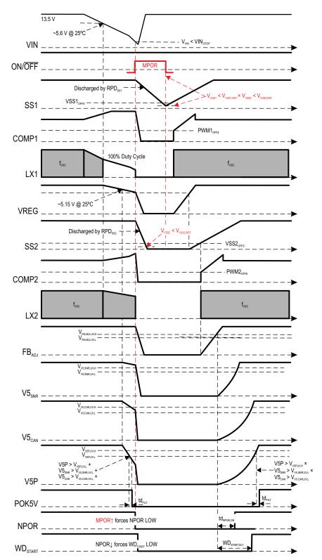
Figure 13: Input Voltage (VIN) Undervoltage, V<sub>VIN</sub> < VIN<sub>STOP</sub> × is for "and", + is for "or"
