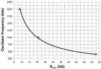
Figure 8: Switching Frequency vs. FSET Resistor
