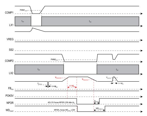
Figure 14: VREG and  $FB_{ADJ}$  Overvoltage Operation
