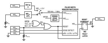
Figure 6: Pulse-Width Window Watchdog
