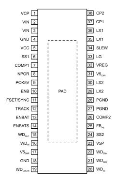
Package LV, 38-Pin eTSSOP Pinout Diagram
