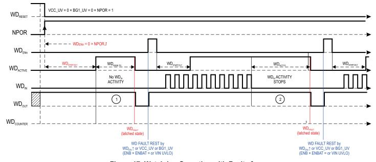
Figure 17: Watchdog Operation with Faults from:
