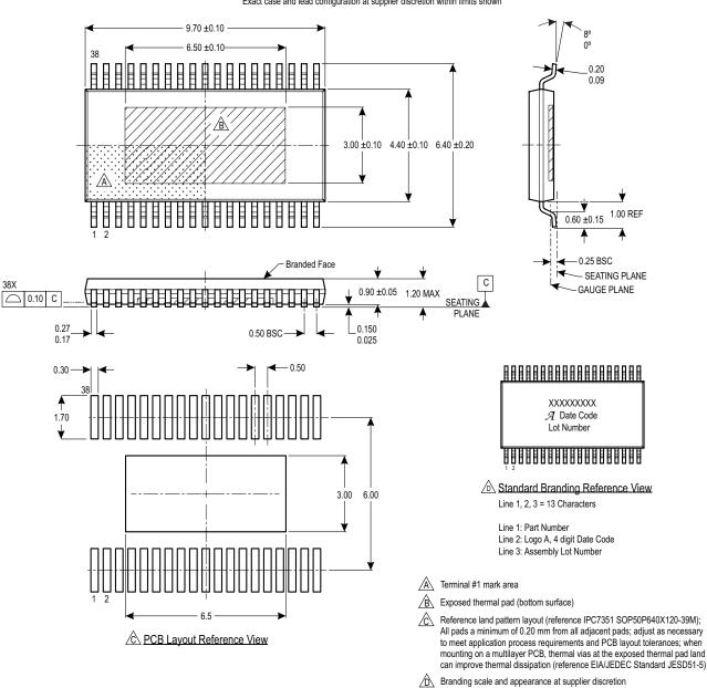
Figure 35: Package LV, 38-Pin eTSSOP
