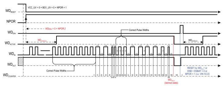
Figure 16: Watchdog (WD) Operation with Both Correct and Incorrect Pulse Widths
