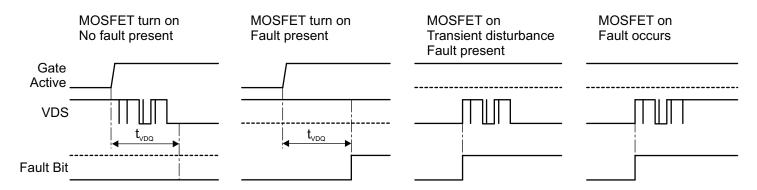
Figure 6: VDS Fault Monitor – Blank Mode Timing (VDQ = 1)
