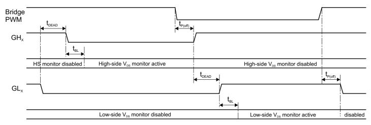
Figure 5: VDS Fault Monitor – Blank Mode Timing (VDQ = 1)
