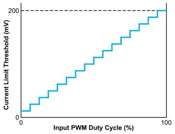
Figure 16: Current Demand vs. Input PWM
