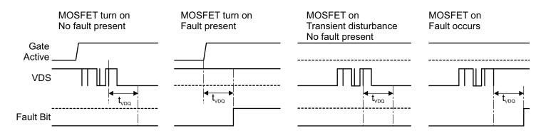
Figure 7: VDS Fault Monitor – Debounce Mode Timing (VDQ = 0)
