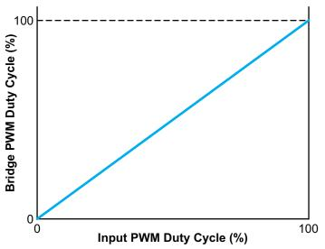
Figure 13: Bridge PWM vs. Input PWM
