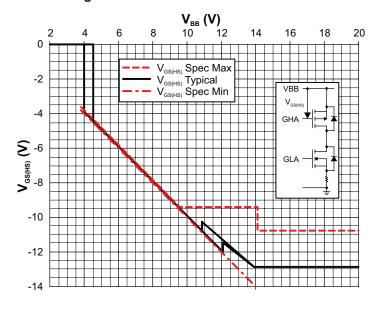
Figure 4: Typical High-Side Gate Drive vs. V<sub>BB</sub>
