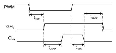
Figure 2: Gate Drive Timing
