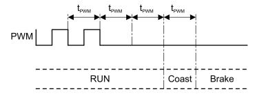
Figure 15: PWM Brake Timing - Indirect Mode PWM
