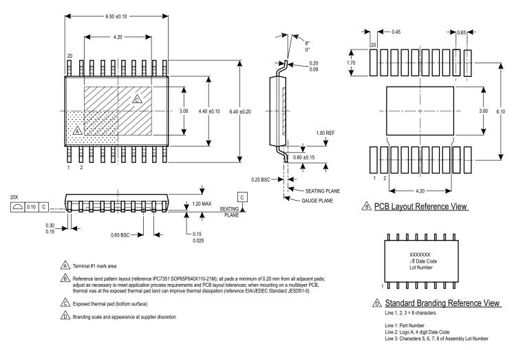
Figure 24: Package LP, 20-Pin TSSOP with Exposed Pad
