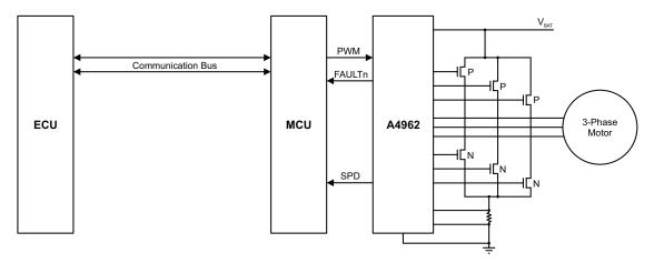
Figure 8: Local Closed-Loop Control with High Level ECU Communications
