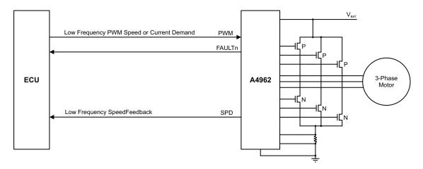
Figure 9: Remote Closed-Loop Control
