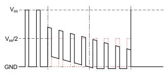
Figure 18c: Low-Side Recirculation, bemf Falling
