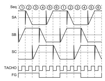
Figure 11: Motor Phase State Sequence
