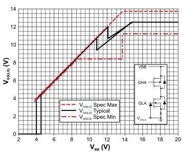
Figure 3: Typical Low-Side Gate Drive vs. V<sub>BB</sub>
