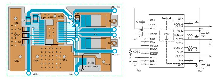
LP Package Typical Application and Circuit Layout
