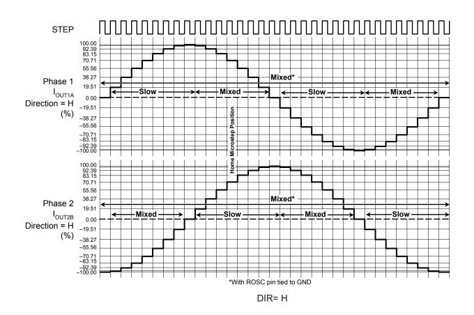
Figure 11: Decay Modes for Eighth-Step Increments
