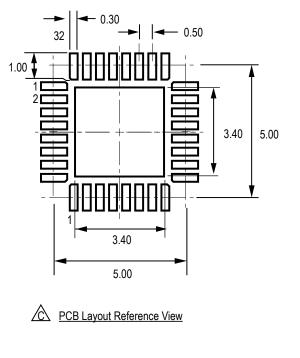
For Reference Only; not for tooling use (reference DWG-0000378, Rev. 3) **Dimensions in millimeters** Exact case and lead configuration at supplier discretion within limits shown
