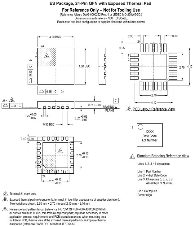
Coplanarity includes exposed thermal pad and terminals
