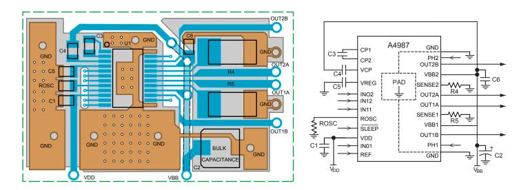
LP package typical application and circuit layout
