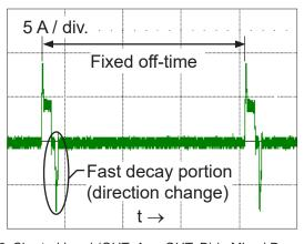
Figure 6: Shorted Load (OUTxA → OUTxB) in Mixed Decay Mode
