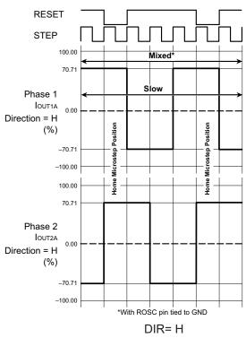
Figure 9: Decay Mode for Full-Step Increments
