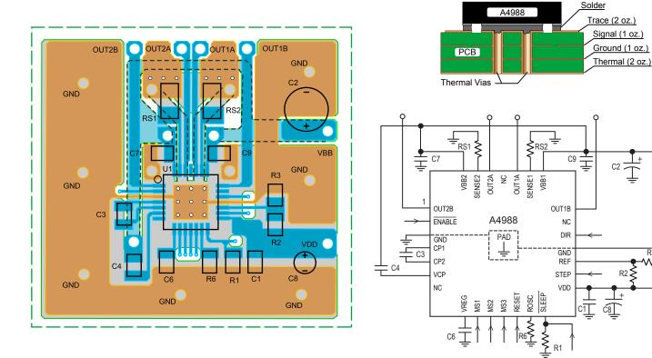
Figure 8: Typical Application and Circuit Layout
