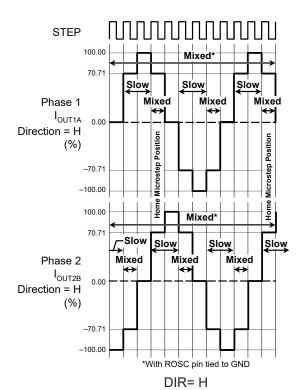
Figure 10: Decay Modes for Half-Step Increments
