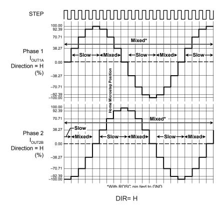
Figure 11: Decay Modes for Quarter-Step Increments
