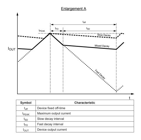
Figure 7: Current Decay Modes Timing Chart
