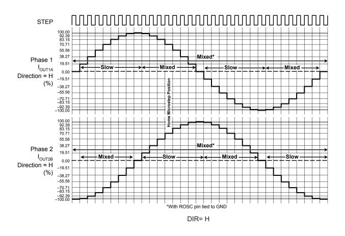
Figure 12: Decay Modes for Eighth-Step Increments
