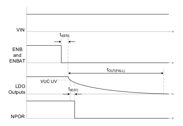
All LDO outputs start to decay  $t_{d(\mathrm{EN})}$  seconds after ENB and ENBAT are low.
