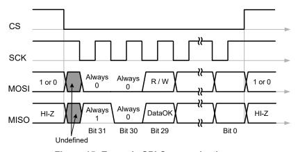
Figure 15: Example SPI Communications
