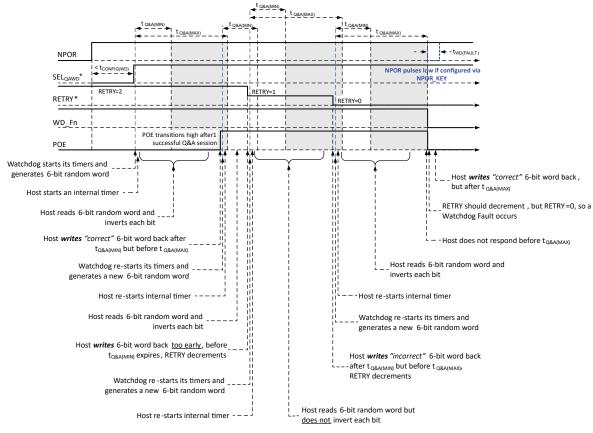
Figure 11: Q&A Selection, Operation, and Fault Examples.
