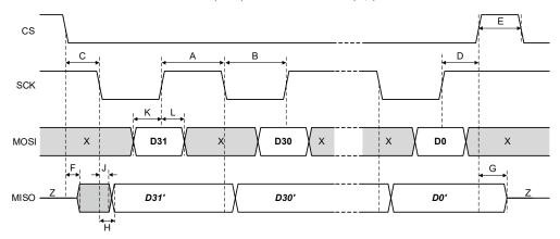
Figure 1: Serial Interface Timing for Write and Read Cycles MISO activity assumes the Chip\_ID from the previous frame was correct
