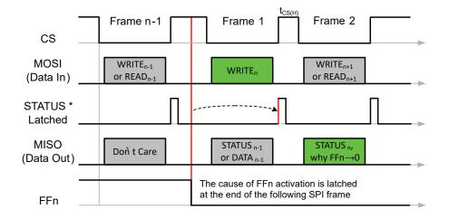
Figure 16: Recommended SPI Operations after FFn→0
