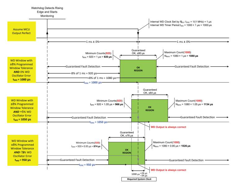
Figure 8: Typical Watchdog Timer System Level Functionality (times are not to scale)
