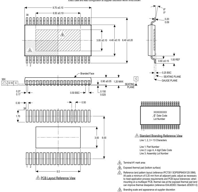
Figure 20: Package LV, 38-Pin eTSSOP
