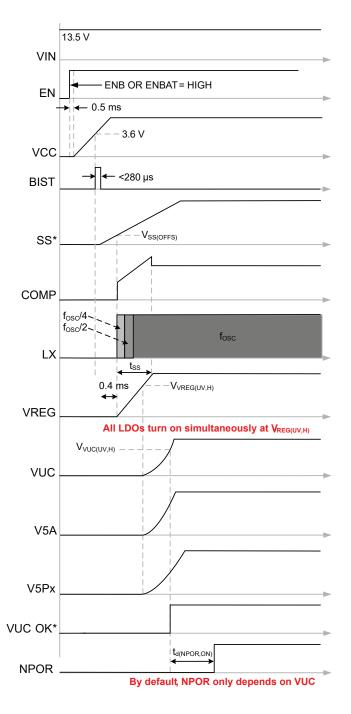
**Figure 2: Startup Timing Diagram**
