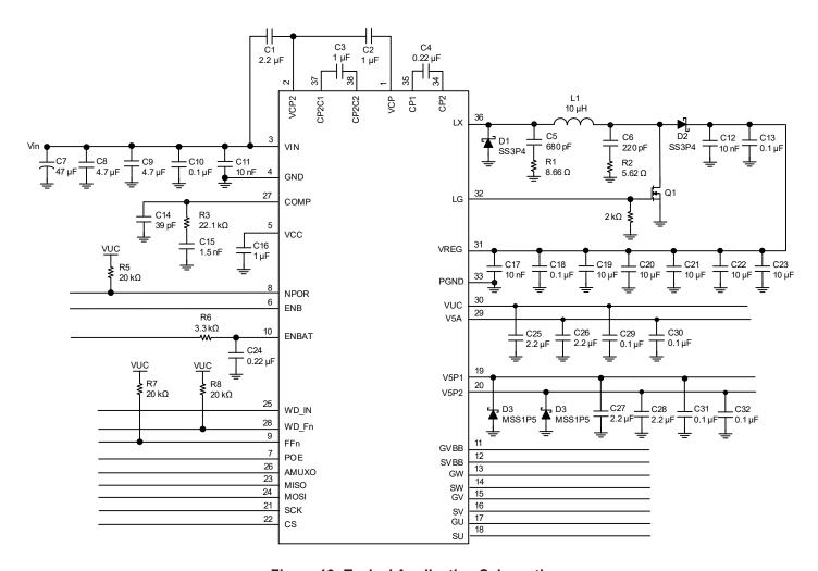
Figure 19: Typical Application Schematic
