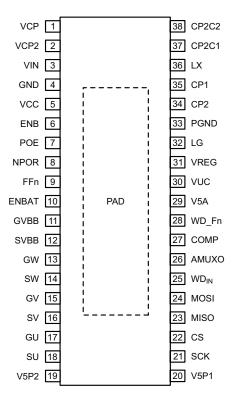
Package LV, 38-Pin eTSSOP Pinout Diagram
