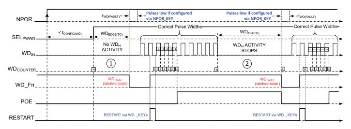
Figure 7: Watchdog operation with faults from:
