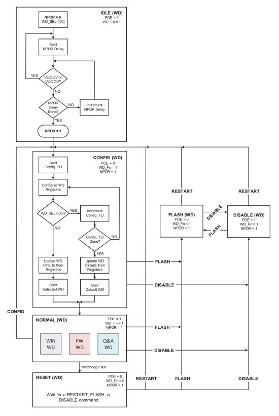
Figure 12: State Diagram of Watchdog Operation
