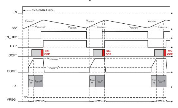
Figure 4: Hiccup Mode Operation with VREG Shorted to GND ( $R_{LOAD}$  < 50 m $\Omega$ )
