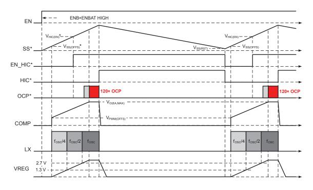
Figure 5: Hiccup Mode Operation with VREG Overloaded ( $R_{LOAD} \approx 0.5 \Omega$ )
