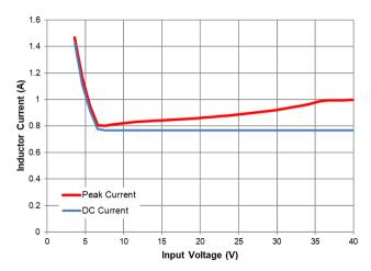
Figure 18: Typical Peak Inductor Current versus Input Voltage for 0.765 A Output Current and 10 µH Inductor
