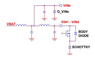
Figure 18. VINS isolated from VIN1/2/3/4, so the addition of  $\mathsf{D}_{\text{VINS}}$  is required
