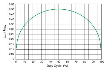
Figure 23. Input capacitor ripple versus duty cycle
