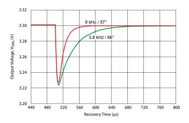
Figure 28. Transient recovery comparison for  $f_{Z2}$  at 3.8 kHz /  $66^\circ$  and 9 kHz /  $57^\circ$
