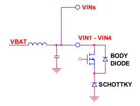
Figure 17. VINS pin connected directly to VIN1/2/3/4 pins
