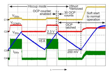
Figure 20. Hiccup mode and recovery to V<sub>SWx</sub> = 3.3 V at I<sub>SWx</sub> = 1.6 A; shows V<sub>SWx</sub> (ch1, 2 V/div), V<sub>COMPx</sub> (ch2, 2 V/div), V<sub>SSx</sub> (ch3, 1 V/div), I<sub>SSSUx</sub> (ch4, 2 A/div); t = 2 ms/div
