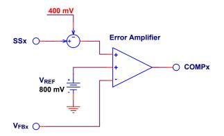
Figure 9. An A8600 error amplifier
