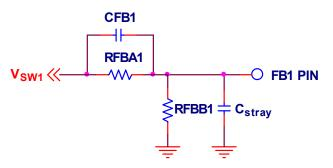
Figure 22. Addition of CFB1 to cancel stray capacitance
