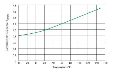
Figure 10. Typical MOSFET R<sub>DS(on)</sub> versus temperature
