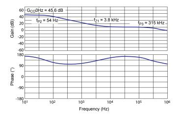
Figure 26. Compensated error amplifier Bode plot (SW3)
