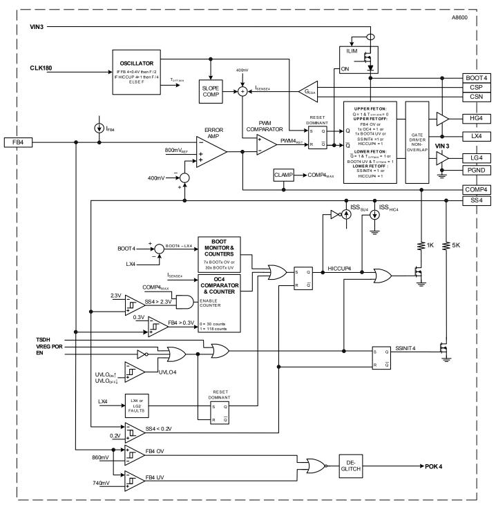
Figure 3. Detailed functional block diagram for SW4
