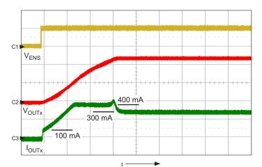
Figure 16. S1/S2 OUTx turning on with a load of 40  $\Omega$  and 22  $\mu$ F; shows V<sub>ENS</sub> (ch1, 5 V/div.), V<sub>OUTx</sub> (ch2, 5 V/div.), I<sub>OUTx</sub> (ch3, 200 mA/div.), t = 500  $\mu$ s/div.
