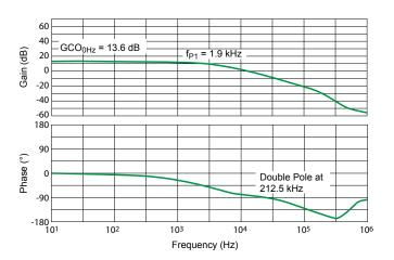
Figure 25. Control-to-output Bode plot for SW3
