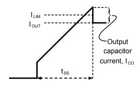
Figure 24. Output current ( $I_{CO}$ ) during startup
