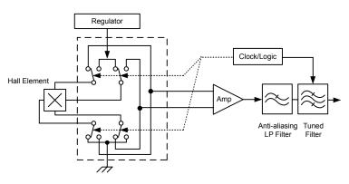
Figure 6. Chopper Stabilization Technique
