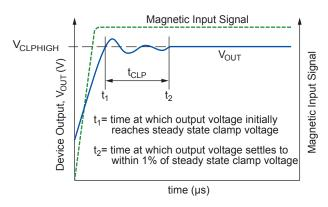
Figure 2. Definition of Delay to Clamp, t<sub>CLP</sub>
