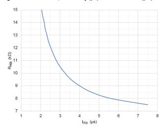
Figure 27: PEB resistor versus PEB delay time.
