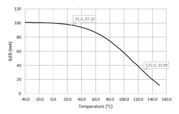
Figure 36: LED current varies with temperature when using thermistor NTCS0805E3684JXT for thermal foldback
