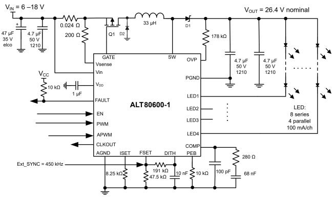
Figure 50: ALT80600-1 Design Example Schematic
