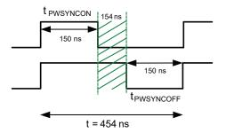
Figure 13: Pulse width requirements for an External Sync clock at 2.2 MHz
