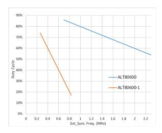
Figure 19: CLKOUT Duty Cycle vs. External Sync Frequency
