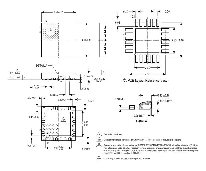
Figure 48: Package ES, 24-Pin 4 mm × 4 mm QFN with Exposed Thermal Pad and Wettable Flank
