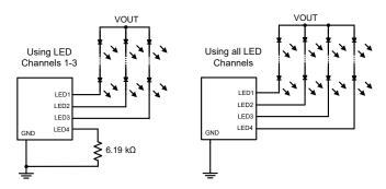
Figure 6: How to signal an unused LED channel during startup LED detection phase
