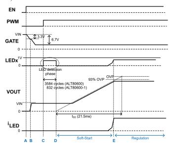
Figure 10: Complete startup process of ALT80600
