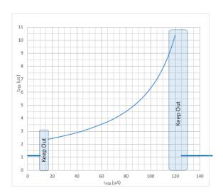
Figure 26: ALT80600-1, PEB Delay (µs) vs. PEB Current (µA).
