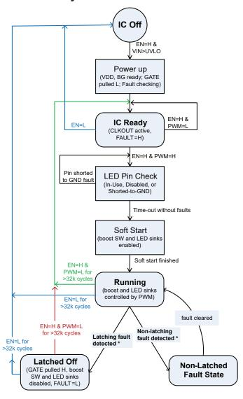
\* Note: Fault conditions may be detected in any state or during any state transition. Most faults are non-latching, meaning the IC will auto-restart as soon as the fault is removed. Only the following faults are latching:
