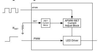
Figure 29: Simplified block diagram of APWM function
