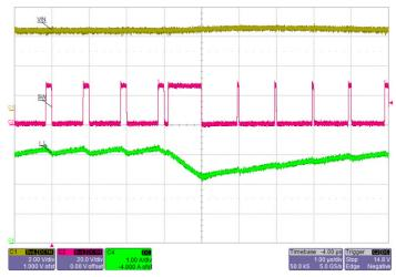
Figure 44: When peak current in SW pin reaches ~3.2 A, overcurrent protection kicks in and the IC skips a switching cycle.
