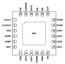
Package ES, 24-Pin QFN Pinouts
