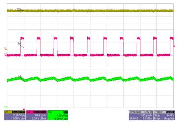
Figure 43: Normal switching waveform showing the SW node voltage and inductor current.
