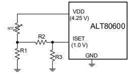
Figure 35: Thermal foldback of LED current using NTC thermistor
