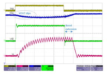
Figure 23: Traditional PWM Dimming operation where boost switch and LED current are enabled at the same time. Note that V<sub>OUT</sub> shows overall ripple of ~0.5 V
