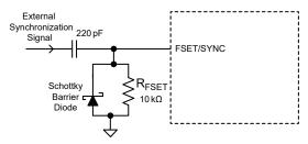
Figure 15: Countermeasure for External Sync Stuck-at-Low Fault
