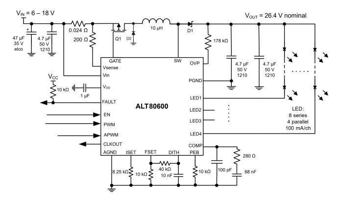
Figure 49: ALT80600 Design Example Schematic
