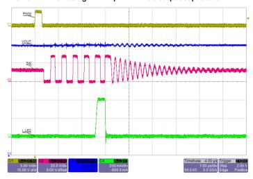
Figure 22: Zoom-in view showing ALT80600 is able to regulate LED current at PWM on-time down to 300 ns.
