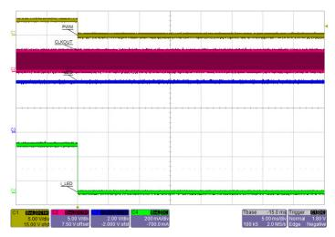
Figure 38: As long as EN = H, the IC does not shut down VDD and CLKOUT. But internal latched faults are cleared by PWM = L for 32k clock cycles (8k cycles for ALT80600-1).
