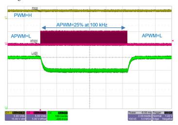
Figure 31: PWM = H. Total LED current drops from 400 mA (4 × 100 mA/ch) to 300 mA when APWM of 25% duty cycle is applied. Note that LED current takes ~0.5 ms to settle after change in APWM.
