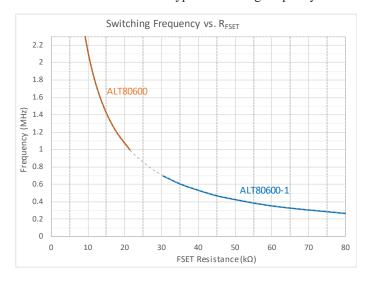
Figure 12: ALT80600 Switching Frequency as a function of FSET Resistance
