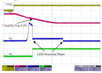
Figure 5: Startup showing EN+PWM, GATE, LED1, and ISET. Switching frequency = 2.15 MHz. Note that LED Detection Phase starts as soon as GATE pin is pulled down to 3.3 V below  $V_{\text{IN}}$ .
