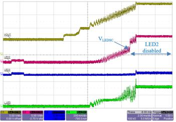
Figure 40: Startup sequence when LED string#2 has a partial-short fault (4 × WLED instead of 6). As soon as LED2 pin rises above  $V_{\rm LEDSC}$  (~4.6 V), the channel is disabled. Output is now 300 mA.
