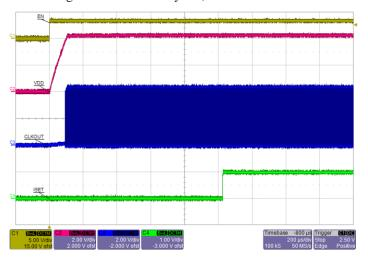
Figure 4: Startup showing EN, VDD, CLKOUT, and ISET (PWM = L). Note that CLKOUT is available as soon as  $V_{DD}$  ramps up, even though Boost stage and LED drivers are not yet enabled.
