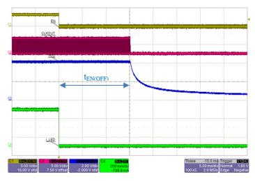
Figure 37: After EN = L for 32k clock cycles (~15 ms at 2.15 MHz), the IC completely shuts down so VDD (Blue) decays.
