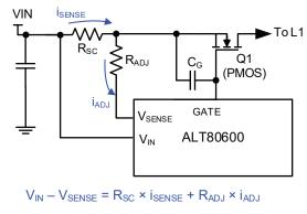
Figure 45: Optional input disconnect switch using a PMOSFET
