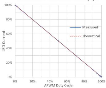
Figure 30: Showing LED current is inversely proportional to the APWM duty cycle. Test conditions:  $V_{IN}$  =12 V,  $V_{OUT}$  = 25 V (8 × WLED), total LED current = 100 mA × 4, APWM frequency = 100 kHz
