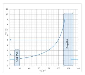
Figure 25: ALT80600 AC, PEB Delay (μs) vs. PEB Current (μA).
