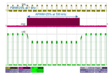
Figure 32: PWM = 25% at 1 kHz. Peak LED current drops from 400 mA (4 × 100 mA/ch) to 300 mA when APWM of 25% duty cycle is applied
