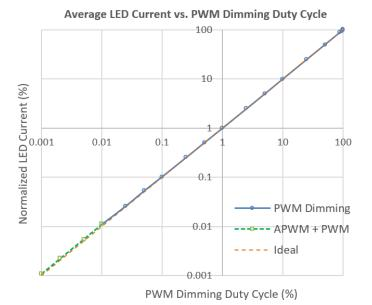
Figure 33: How to achieve 100,000:1 dimming ratio by using both PWM and APWM. Test conditions:  $V_{IN}$  = 12 V,  $V_{OUT}$  = 25 V (8 × WLED), total LED current = 400 mA, PWM frequency = 200 Hz, APWM frequency = 100 kHz.
