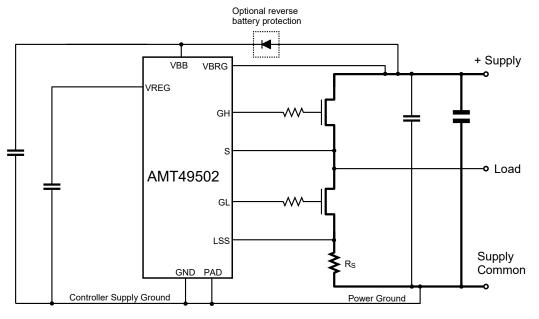
Figure 10: Supply Routing Suggestions
