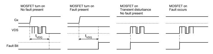
Figure 6a: VDS Fault Monitor – Blank Mode Timing (VDQ = 1)
