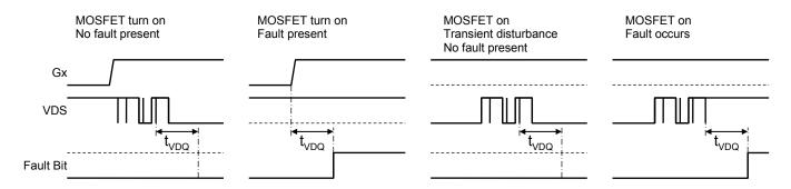
Figure 6b: VDS Fault Monitor – Debounce Mode Timing (VDQ = 0)
