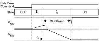
Figure 8a: Off-to-On Transition (Gate Drive)
