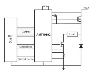
Figure 7: PWM Load current control
