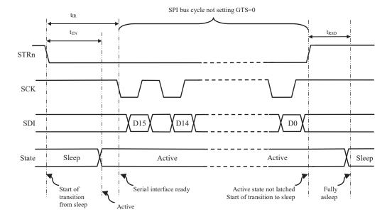
Figure 4c: Transition from Sleep (SPI, Active State Not Latched)
