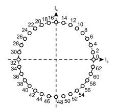
Figure 14: Eighth-Step Phase Diagram
