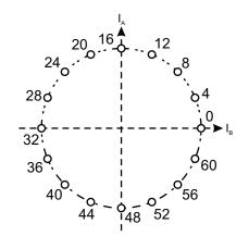
Figure 13: Quarter-Step Phase Diagram
