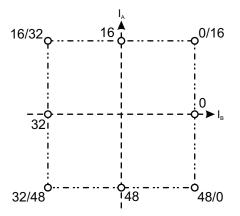
Figure 12: Uncompensated Half-Step Phase Diagram
