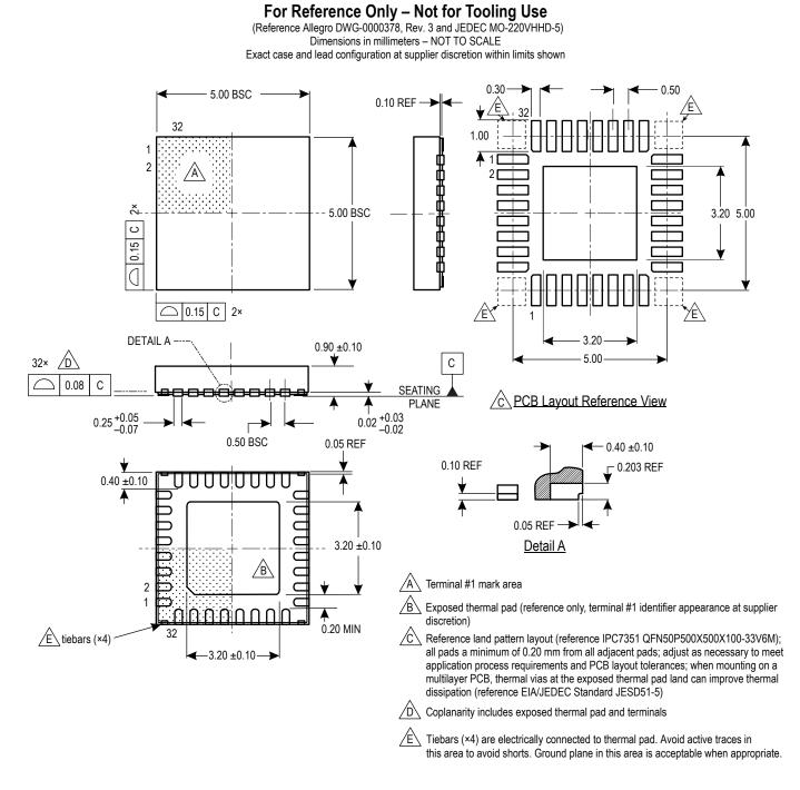
Figure 26: Package ET, 32-Pin QFN with Exposed Pad and Wettable Flank
