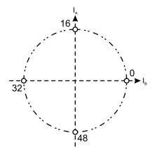
Figure 9: Full-Step 1-Phase Drive Phase Diagram
