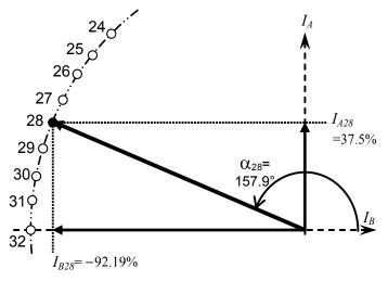
Figure 7: Calculating the Resultant Motor Current
