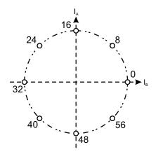
Figure 11: Compensated Half-Step Phase Diagram
