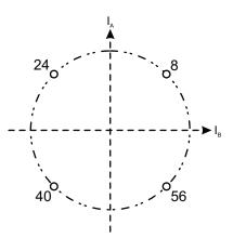
Figure 10: Full-Step 2-Phase Drive Phase Diagram
