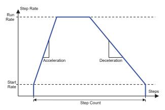
Figure 5: Step Profile Parameters
