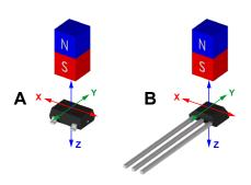
Figure 2: Magnetic Sensing Orientations APS11450 LH (Panel A), APS11450 UA (Panel B)
