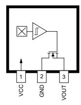
LH Package, 3-Pin SOT23W Pinout
