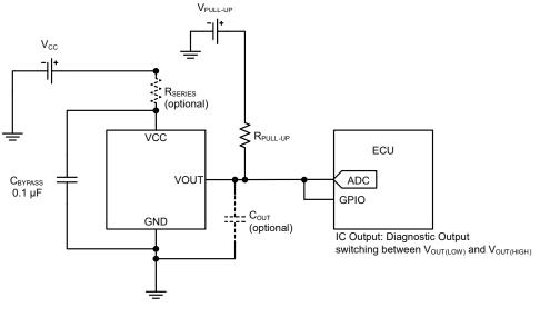
Figure 9: Typical Applications Circuits Diagnostic Output
