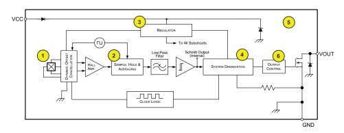
Figure 3: Diagnostics Coverage Block Diagram
