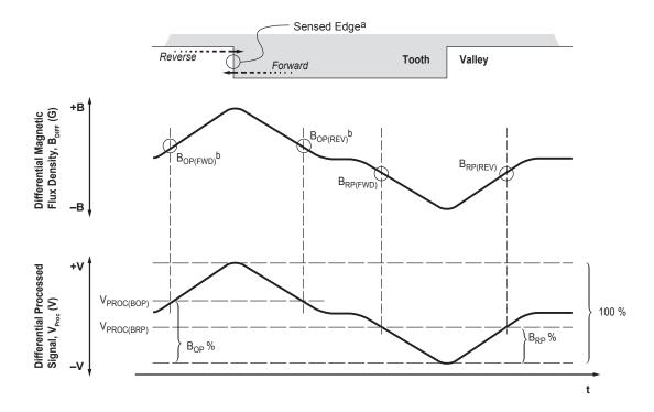
Figure 1: (a) Sensed Edge: leading (rising) mechanical edge in forward rotation, trailing (falling) mechanical edge in reverse rotation; (b) B<sub>OP(FWD)</sub> triggers the output transition during forward rotation, and B<sub>OP(REV)</sub> triggers the output transition during reverse rotation.
