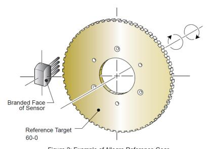
Figure 2: Example of Allegro Reference Gear
