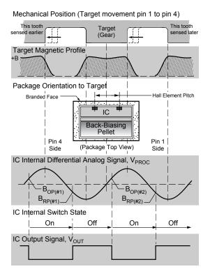
Figure 3. The magnetic profile reflects the geometry of the target, allowing the ATS667 to present an accurate digital output response.
