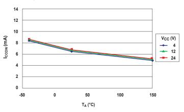
Supply Current (On) versus Supply Voltage
