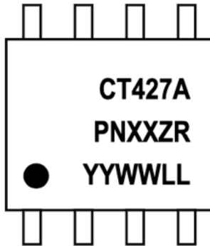
Figure 47: CT427 Device Marking for 8-lead Package
