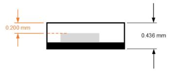
Figure 36: XtremeSense TMR Sensor Location in z Dimension for CT815x in 4-lead LGA Package
