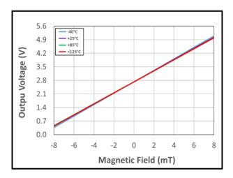
Figure 10: Output Voltage vs. Magnetic Field over Temperature at  $V_{DD}$  = 5.5 V
