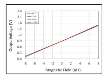
Figure 19: Output Voltage vs. Magnetic Field over Temperature at V<sub>DD</sub> = 1.8 V
