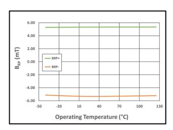
Figure 17: B<sub>RP-</sub> (Orange) and B<sub>RP+</sub> (Green) vs. Temperature at  $V_{DD} = 3.3$  V
