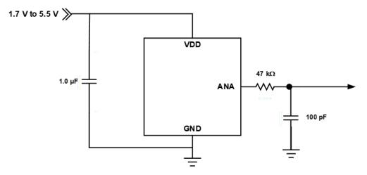
Figure 31: CT8150 Application Block Diagram
