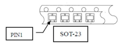
Figure 42: SOT23 Orientation in Tape Pocket
