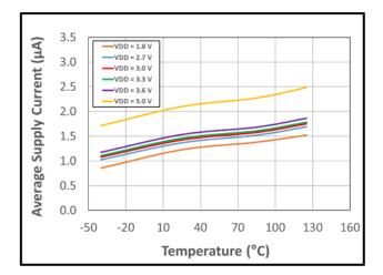
Figure 11: Average Supply Current vs. Supply Voltage vs. Temperature
