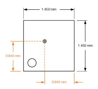
Figure 34: XtremeSense TMR Sensor Location for CT815x products in 4-lead LGA Package
