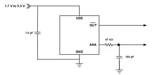
Figure 32: CT8152 Application Block Diagram
