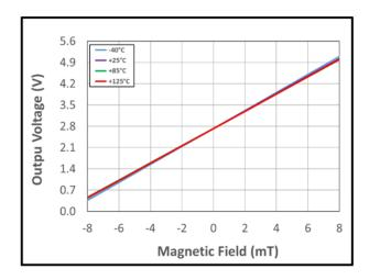
**TYPICAL MAGNETIC CHARACTERISTICS FOR CT8152PC IN ANALOG MODE**
