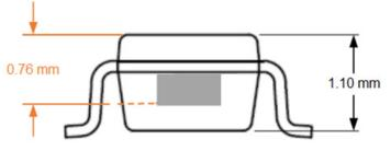
Figure 37: XtremeSense TMR Sensor Location in z Dimension for CT815x in SOT23 Package
