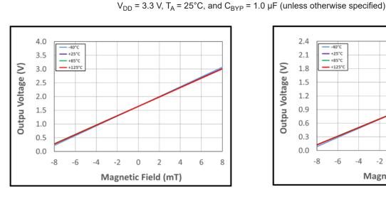
Figure 18: Output Voltage vs. Magnetic Field over Temperature at V<sub>DD</sub> = 3.3 V
