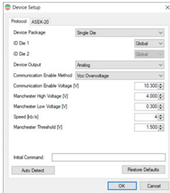
8. Once the Device Setup is finished, the user can power on and communicate with the device.
