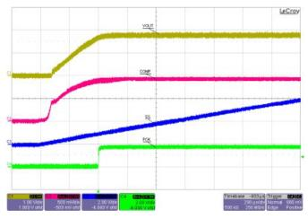
Figure 3: Startup with VIN = 5 V, IOUT = 1.8 A (1  $\Omega$  load)
