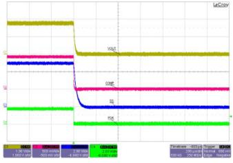
Figure 4: Shutdown with VIN = 5 V, IOUT = 1.8 A (1  $\Omega$  load)
