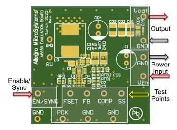
Figure 2: APEK8650 Evaluation Board I/O Connections and Default Jumper Positions
