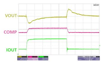
Figure 5: V<sub>OUT</sub> Response to Load Transient with VIN = 5 V and Load Step = 500 mA to 1.5 A
