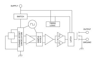
Fig. 24. Chopper-stabilized Hall circuit
