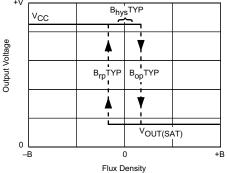
Fig. 8. Bipolar latch or bipolar switch in latch mode
