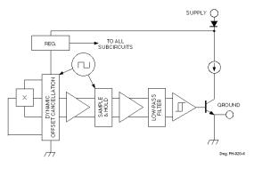
Fig. 10b. Two-wire configuration
