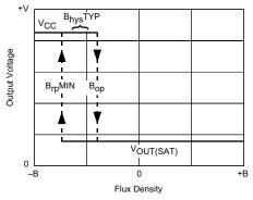
Fig. 9. Bipolar latch, negative unipolar mode
