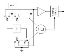
Fig. 22a. Chopper-stabilized Hall circuit
