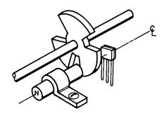
Fig. 17a. Axle-mount vane interrupter
