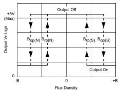
Fig. 7. Omnipolar switch. N, relative to north pole; S, relative to south pole.
