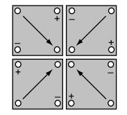
*Fig. 21a. Four-element Hall device (arrows indicate current)*
