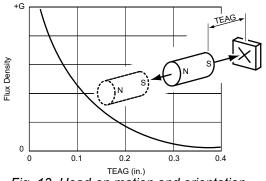
Fig. 13. Head-on motion and orientation
