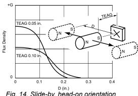
Fig. 14. Slide-by, head-on orientation
