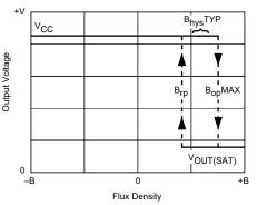
Fig. 6. Unipolar switch or bipolar switch in unipolar mode
