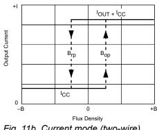
Fig. 11b. Current mode (two-wire)
