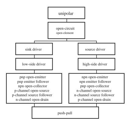
Figure 2 — Hierarchy of unipolar outputs
