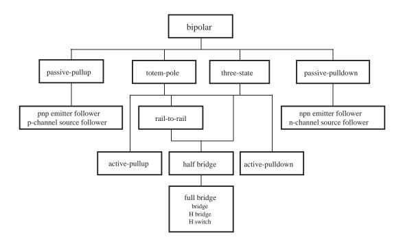
Figure 1 — Hierarchy of bipolar outputs
